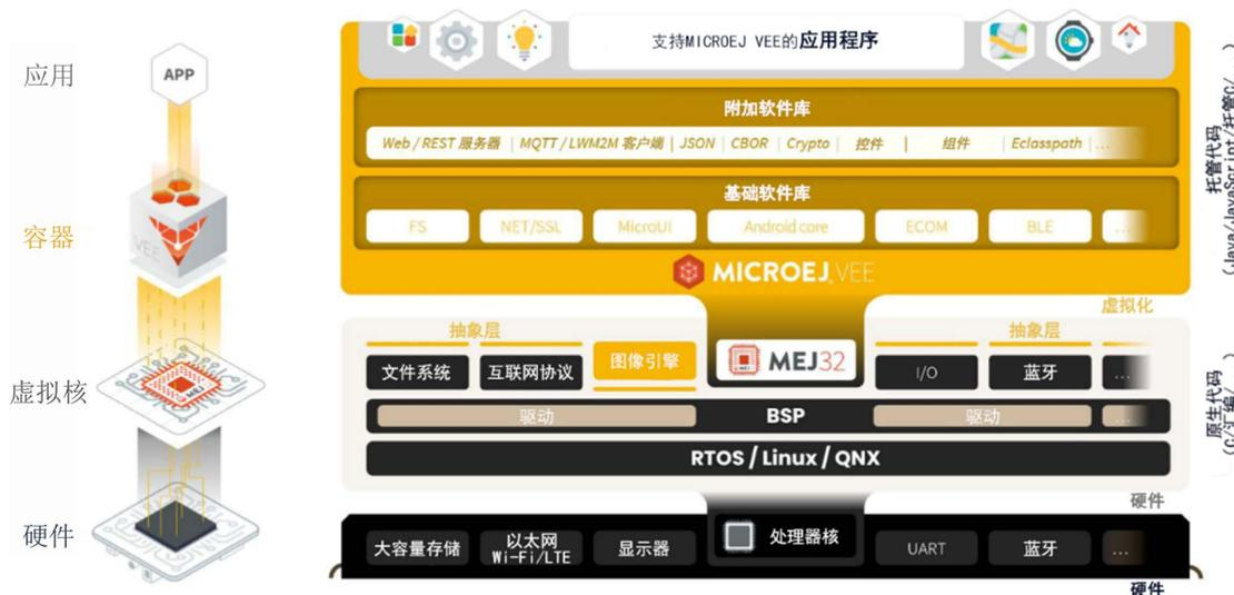
Figure 5. A small real-time container solution: MICROEJ VEE
